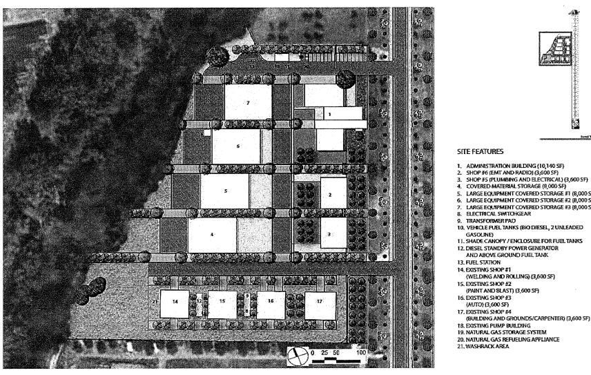
Figure 1. Layout for Proposed Sunol Yard
