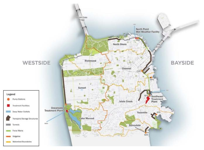
Figure 1-1 – SFPUC Wastewater Enterprise and Major Facilities (Not to Scale)
