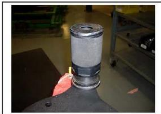
Figure 28 - Suspension Block Locked onto Suspension Plate
