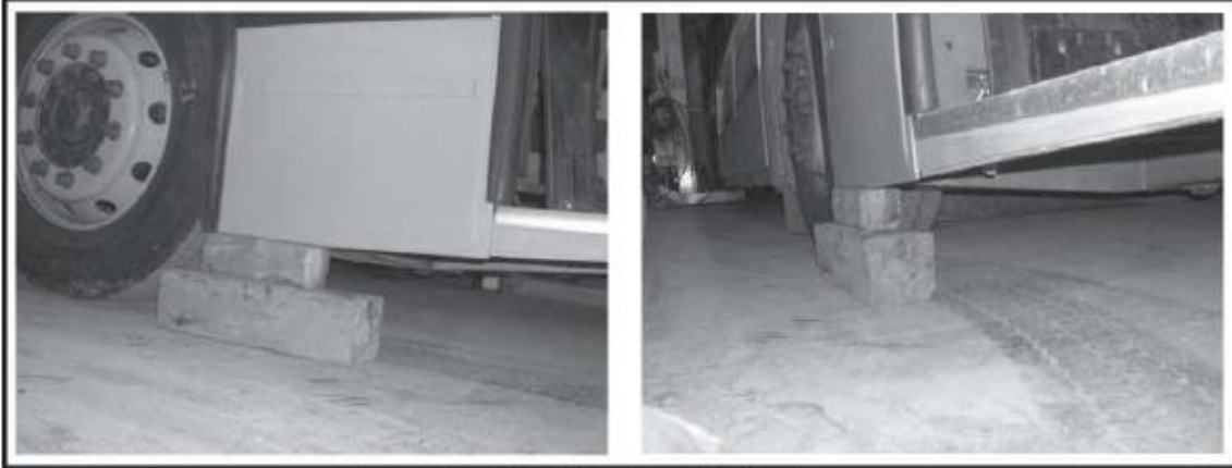
Figure 32 - Positioning of Wood Blocks
