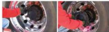
Figure 21-30. Removing the Half Shaft
