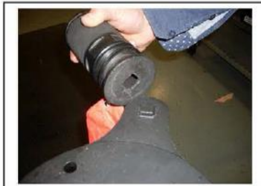
Figure 27 - Suspension Block Fits on Air Suspension Plate
