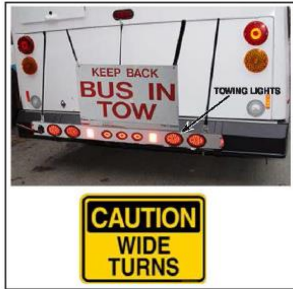
Figure 22 - Safety Towing Lights and Signs Attached to Rear of Vehicle
