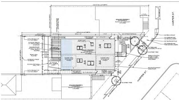
Figure 2. Planned fenestration and skylight changes, 72 Harper St.
