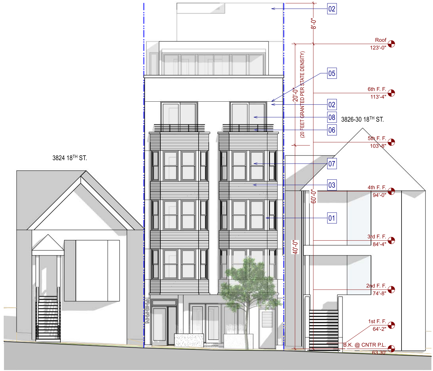
1 Proposed Front Elevation (North) Scale: 3/16" = 1'-0"
