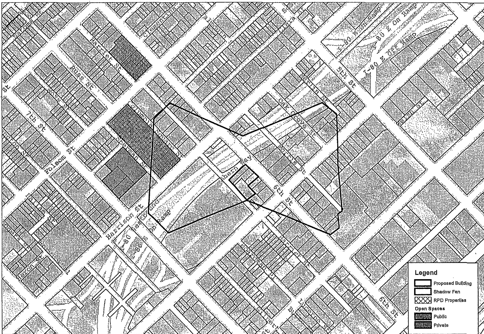
Title: Proposed Rehabilitation and Detention Facility (110 feet with 15-foot mechanical penthouse) Source: San Francisco Planning Department
