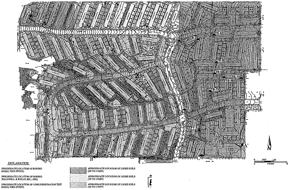
Soil boring site plan: Up to 5' of loose soils are located at the portion of site east of Santos Street. (Figure 1.6)
