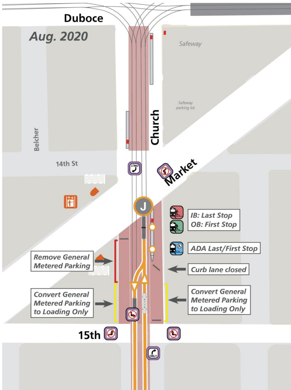
Transfer configuration after proposed construction of a new temporary accessible platform on Church Street between Market and 15th streets
