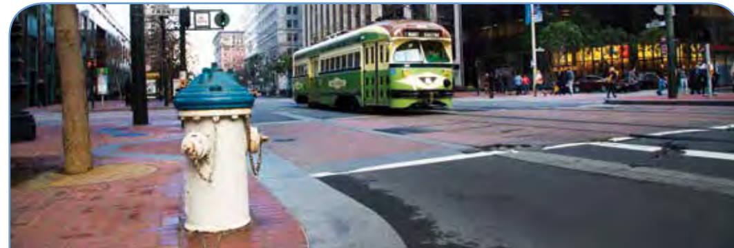
Properly designed bulb-outs and sidewalk extensions enhance pedestrian safety while providing continued access to hydrants and other assets for operation and maintenance.
