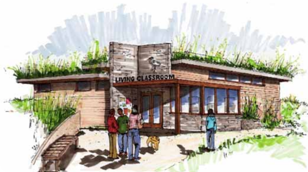
A vegetated roof and other LID features at the Eco-Center at Heron's Head Park help illustrate sustainable design practices to students in San Francisco's Bayview-Hunters Point neighborhood.
