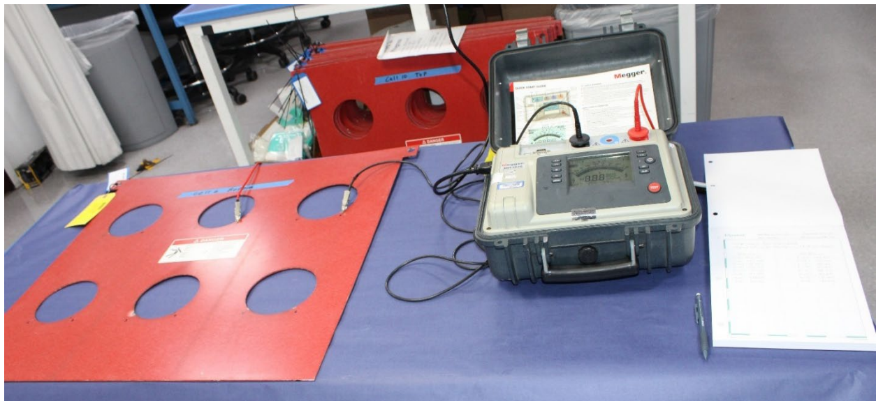
Figure 33. Insulation resistance test set up between selected locations on a barrier insulation board.
