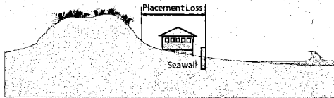
b) Placement loss of beach due to construction of seawall and house
