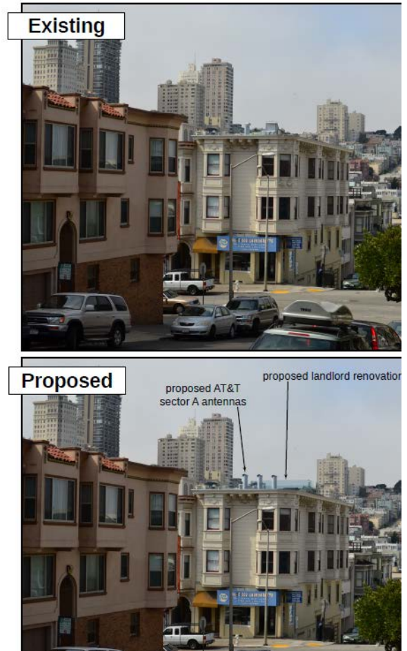
Previously approved AT&T Mobility “Macro” WTS Facility in Telegraph Hill. The facility consists of three (3) faux vent pipes (with a total of three [3] antennas) on the roof, and equipment inside the garage. The initial submittal featured nine (9) vent pipes and was not compatible with the subject building or surrounding neighborhood.
