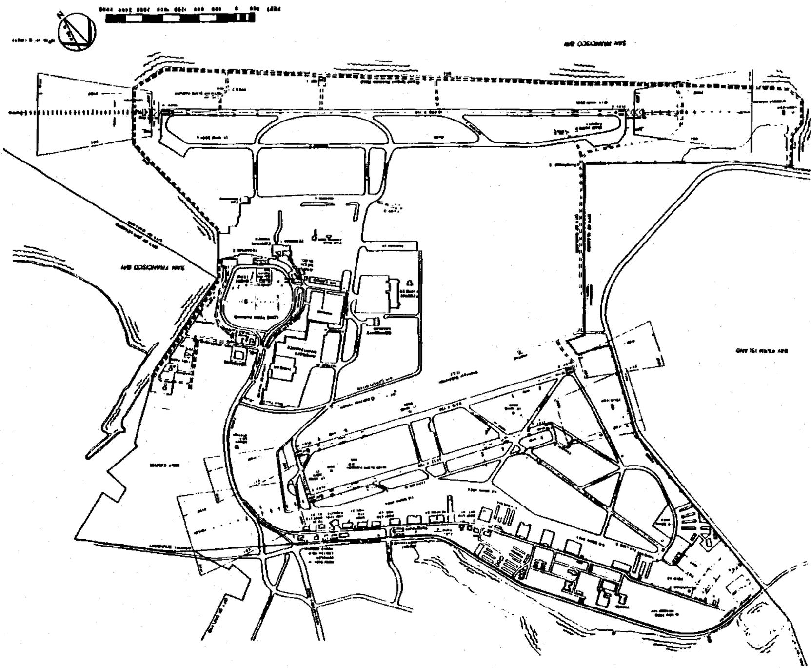
6,212 feet long and 150 feet wide; 9L-27R, which is 5,452 feet long and 150 feet wide; and 15-33, a short crosswind runway which is 3,366 feet long and 75 feet wide. The air carrier runway, 11-29 at South Field is approximately 6,400 feet from the closest general aviation runway, runway 9-27. There is one designated helicopter takeoff/landing area.
