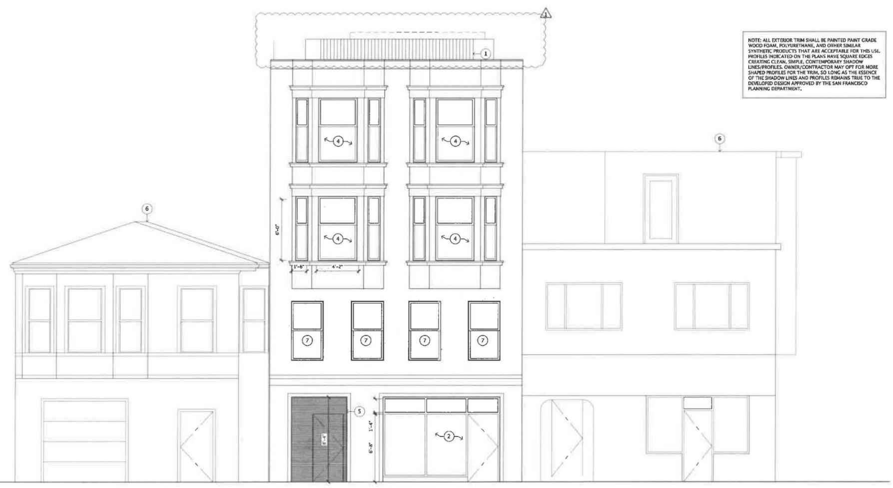
NOTE: ALL EXTERIOR TRIM SHALL BE PAINTED PAINT GRADE WOOD FOAM, POLYURETHANE, AND OTHER SIMILAR SYNTHETIC PRODUCTS THAT ARE ACCEPTABLE FOR THIS USE. PROFILES INDICATED ON THE PLANS HAVE SQUARE EDGES CREATING CLEAN, SIMPLE, CONTEMPORARY SHADOW LINES/PROFILES. OWNER/CONTRACTOR MAY OPT FOR MORE SHARPED PROFILES FOR THE TRIM, SO LONG AS THE ESSENCE OF THE SHADOW LINES AND PROFILES REMAINS TRUE TO THE DEVELOPED DESIGN APPROVED BY THE SAN FRANCISCO PLANNING DEPARTMENT.
