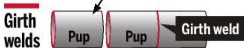
Within the 44-foot section of the damaged pipeline were six smaller pieces, known as "pups," all welded end-to-end at the girth on-site in 1956.
