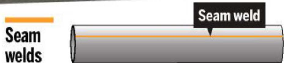
Done at a factory, pipes were made by rolling steel sheets and welding them at the seam. Investigators found numerous welds only penetrated halfway through the steel when they should have gone all the way.
