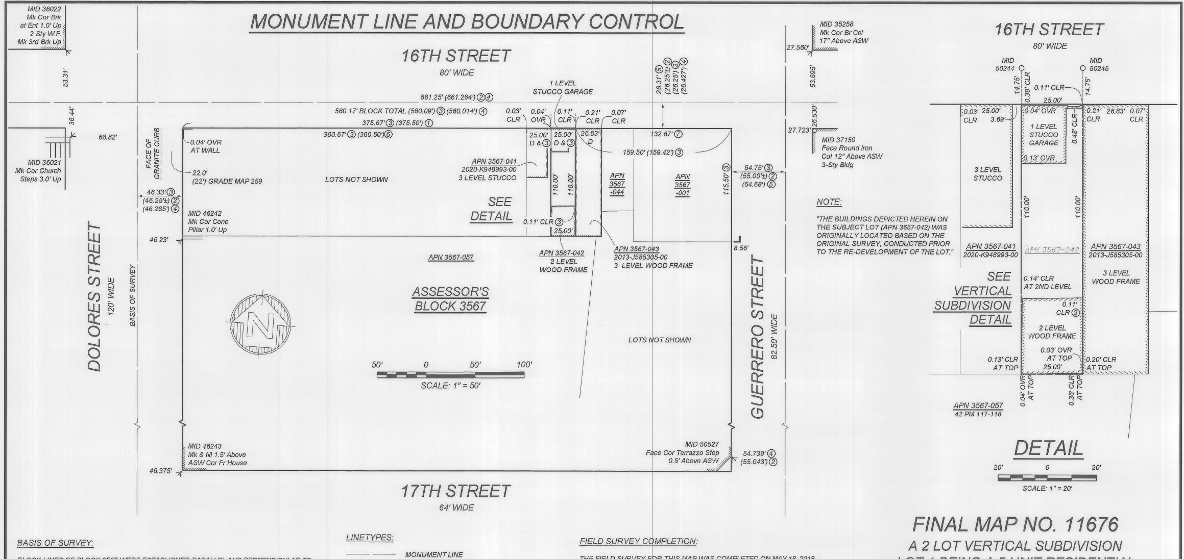
BLOCK LINES OF BLOCK 3567 WERE ESTABLISHED PARALLEL AND PERPENDICULAR TO THE CITY MONUMENT LINE ALONG DOLORES STREET IDENTIFIED AS BASIS OF SURVEY.
