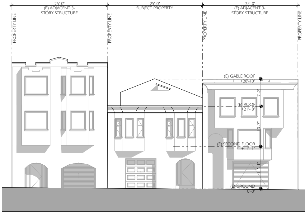
4 (E) EAST (FRONT) ELEVATION SCALE: 1/8" = 1'-0"
