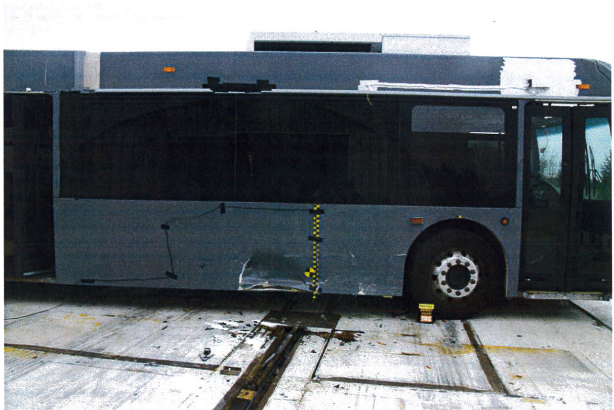
Figure A-8 Post-Test Bus Right Side Close-up View
