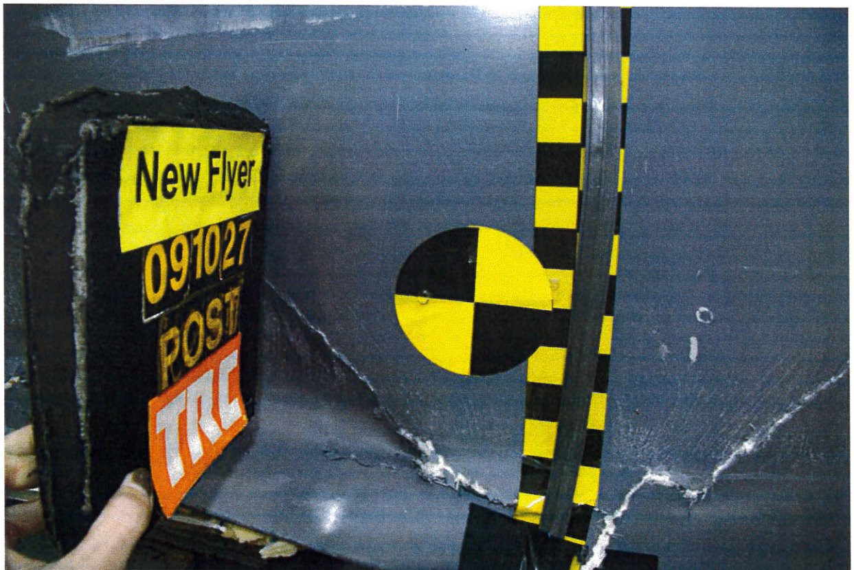
Figure A-25 Post-Test Impact Point Close-up View
