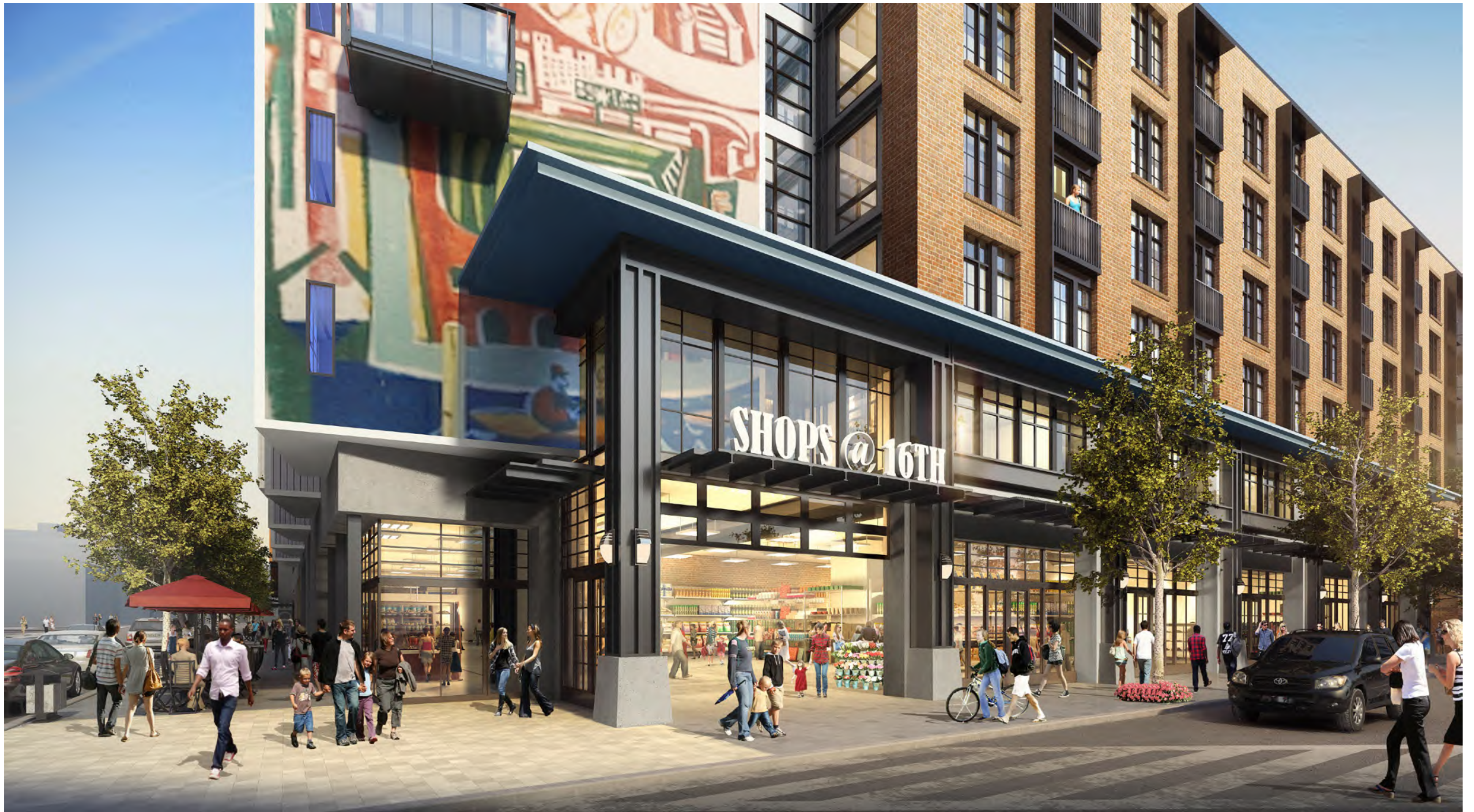
VIEW FROM 16TH ST. LOOKING SOUTH AT RETAIL CORNER ON MISSISSIPPI ST. - TWO LEVEL RETAIL BASE EXPRESSION WITH RECESSED CORNER TO ALLOW FOR A LARGER OUTDOOR ENTRY PLAZA
