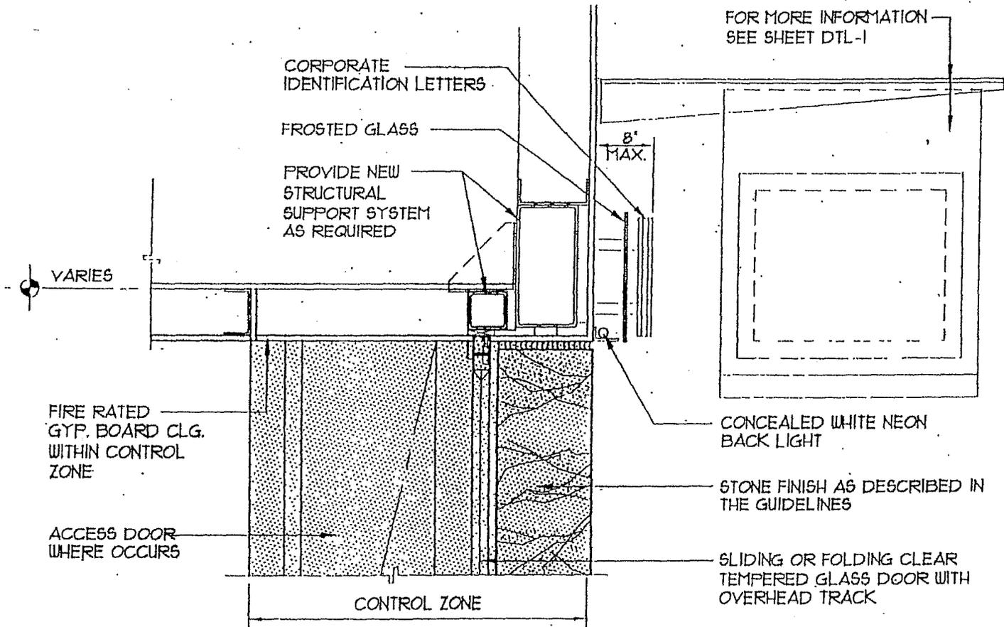
**SOFFIT DETAIL - CONDITION #1**
