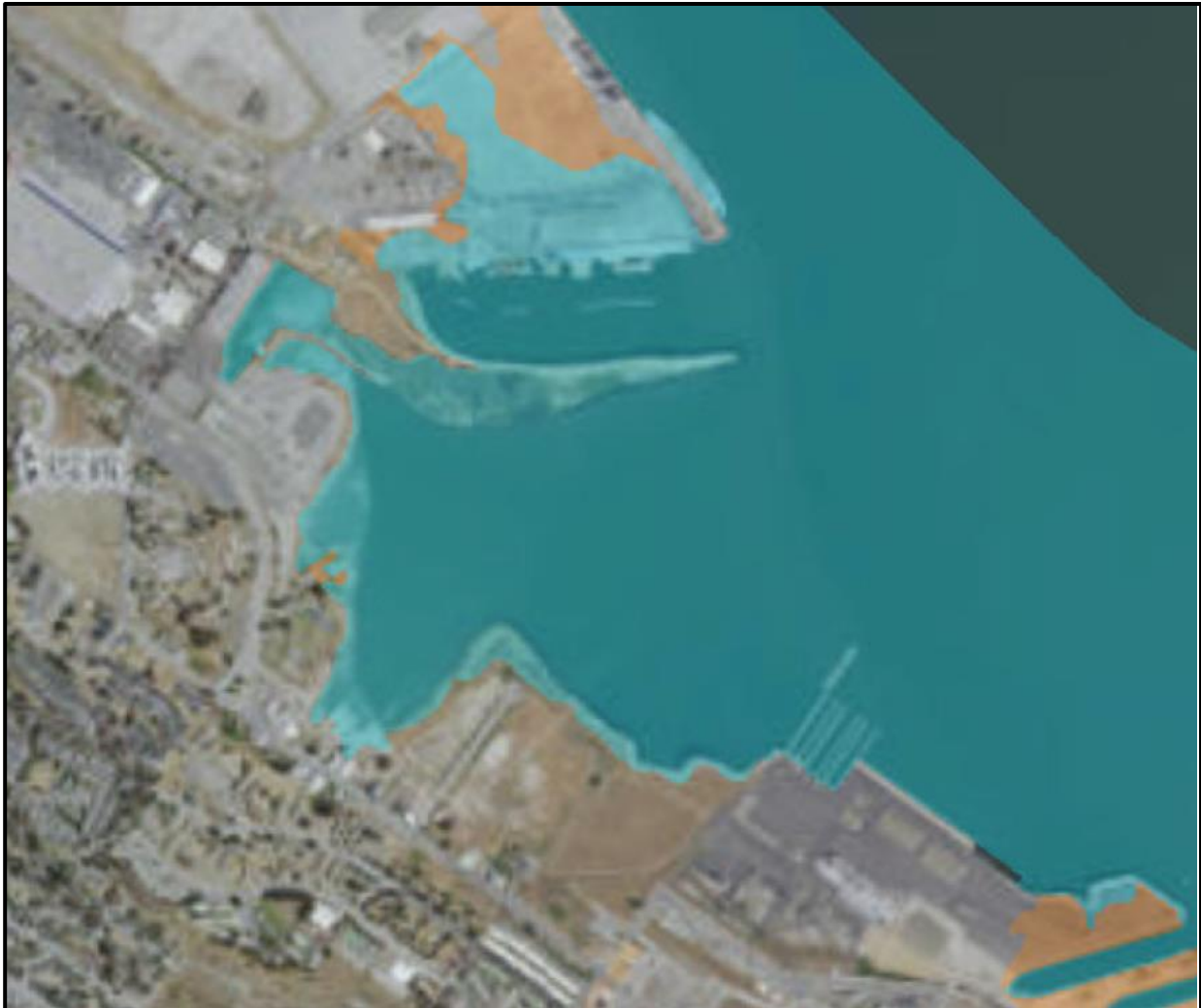
Figure 4-13: Preliminary Flood Insurance Rate Map (FEMA Nov. 2015) 100-year (Blue) and 500-year (Orange).
