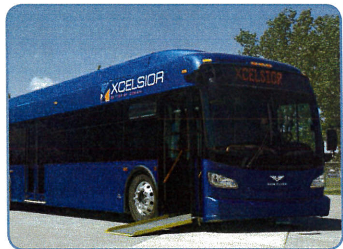
Ramp deployed kneeled (1:7) street level
