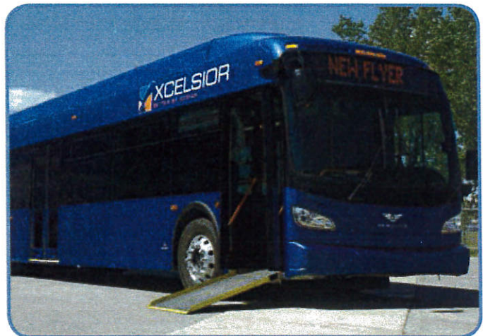
Ramp deployed at ride height street level
