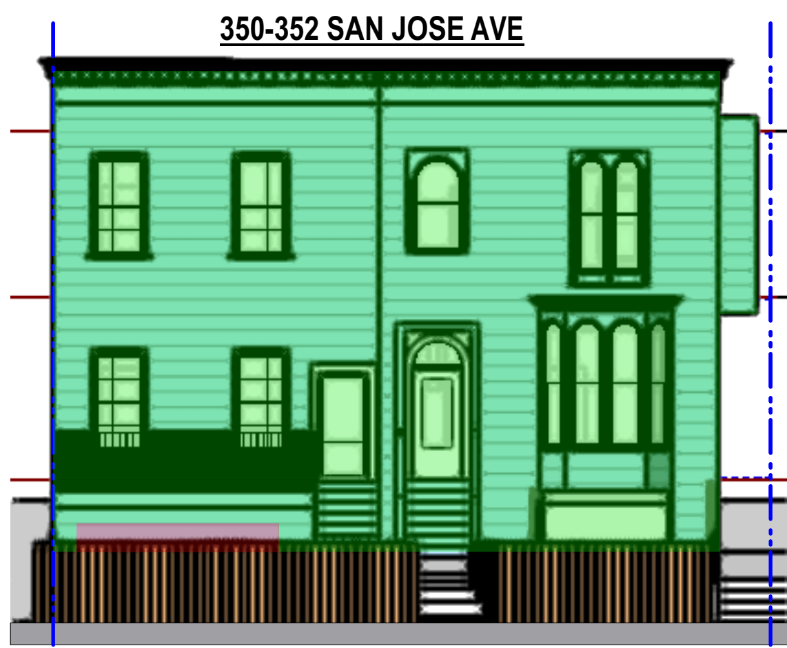
Existing Front Elevation 1/8" = 1'-0"
