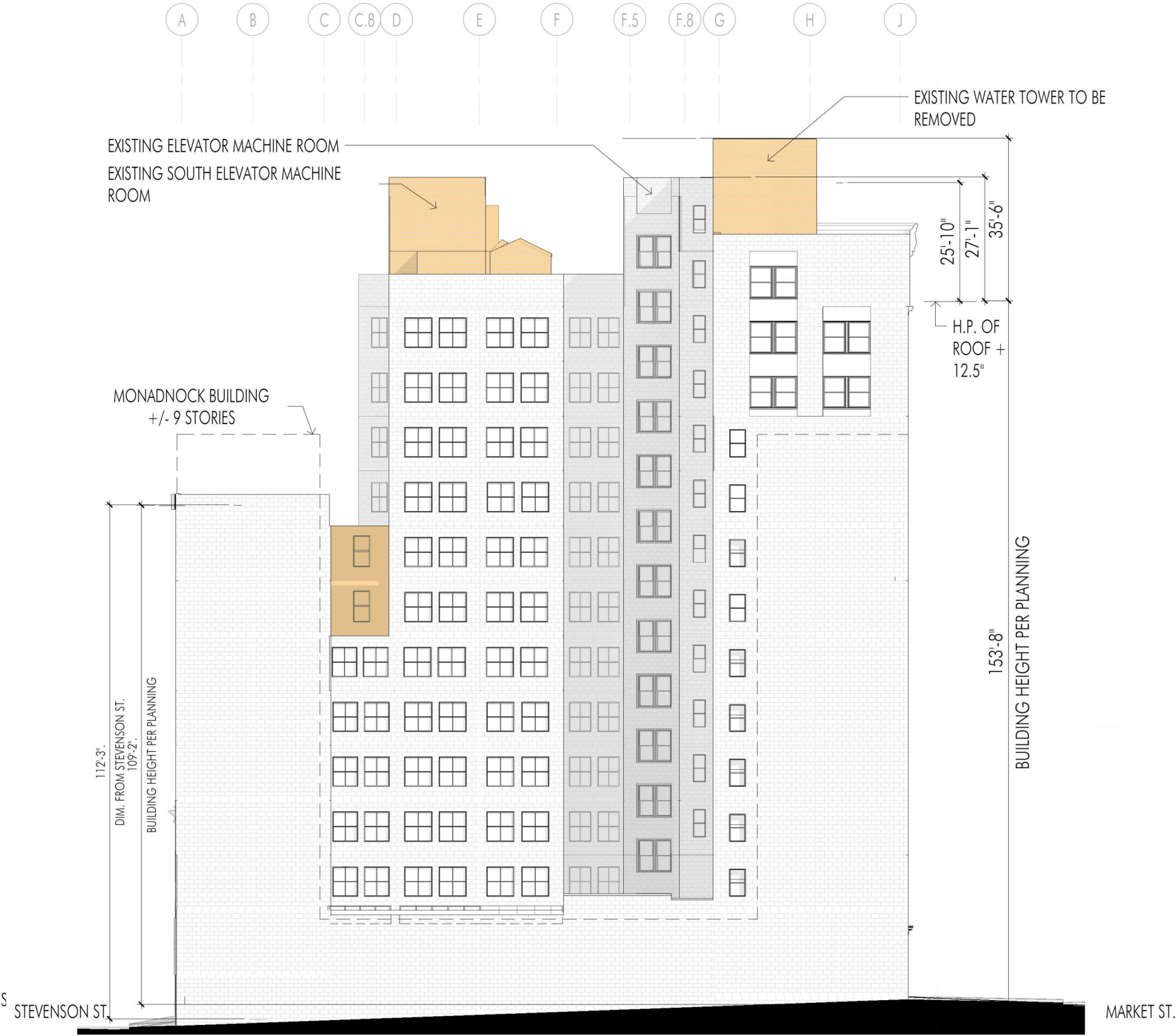
EXISTING COURTYARD ELEVATION
