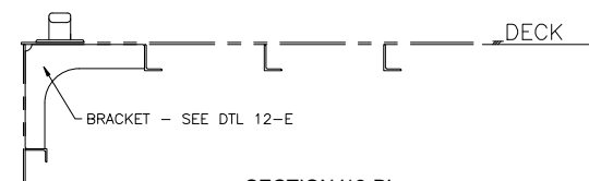
SECTION '12-D' TYPICAL KEVEL FOUNDATION STBD SIDE, PORT SIMILAR, OPP HAND LKG AFT SCALE: 1/2"=1'-0"
