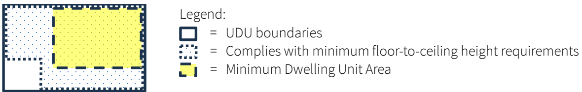
Figure A: Example UDU meeting both the minimum floor-to-ceiling height and minimum area
