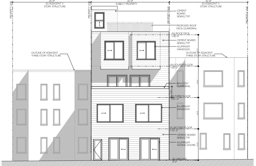
2 (N) PROPOSED WEST (REAR) ELEVATION SCALE: 1/8" = 1'-0"
