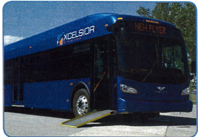
Ramp deployed at ride height street level
