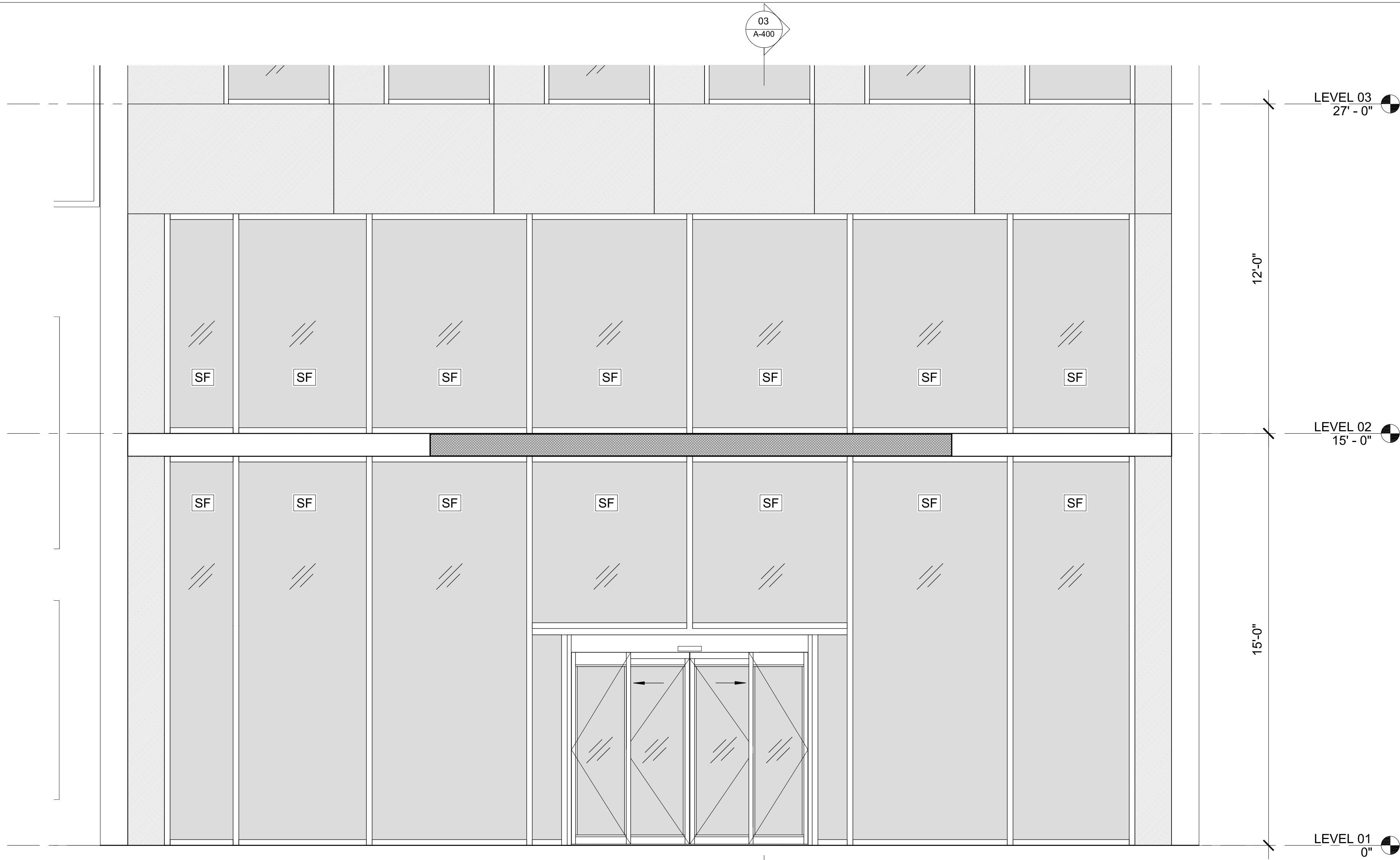
ENLARGED BUILDING ELEVATION - NORTH - ENTRY 3/8" = 1'-0"
