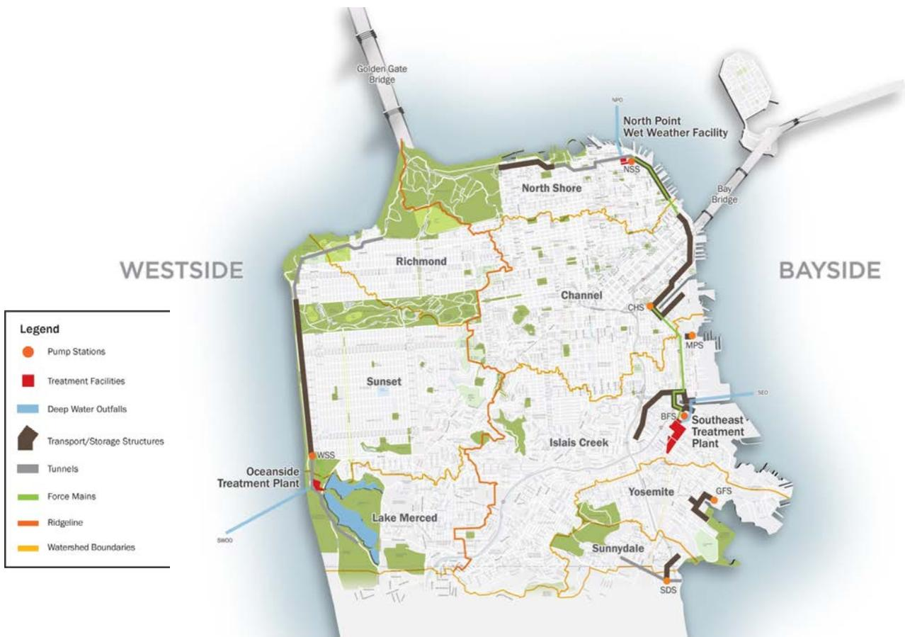
Figure 1-1 – SFPUC Wastewater Enterprise and Major Facilities (Not to Scale)
