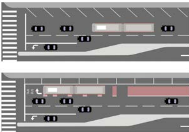
Diagram showing a bus approaching an intersection without transit lanes vs. with transit lanes. It only takes one or two cars to prevent a bus from catching a green light.
