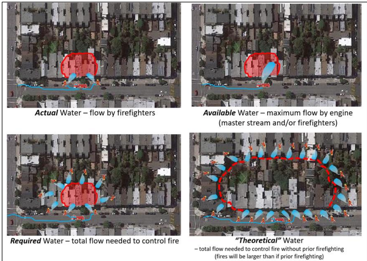
Figure 90 Four categories of water usage: (top left) Actual water, being the water used by available firefighters; (top right) Available water, being the maximum flow by available engines (typ. a master stream); (lower left) Required water, being the total flow required to control the fire, and (lower right) “Theoretical” water, being the total flow at a point in time required to control the fire, if no firefighting has previously occurred (in this last case, the fire will have grown larger than the previous cases).
