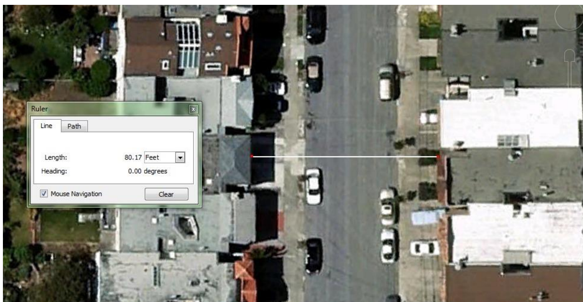
Figure 68 Street width (building face-building face) sampled from Google Earth (example: 27 th Ave between Moraga and Noriega).
