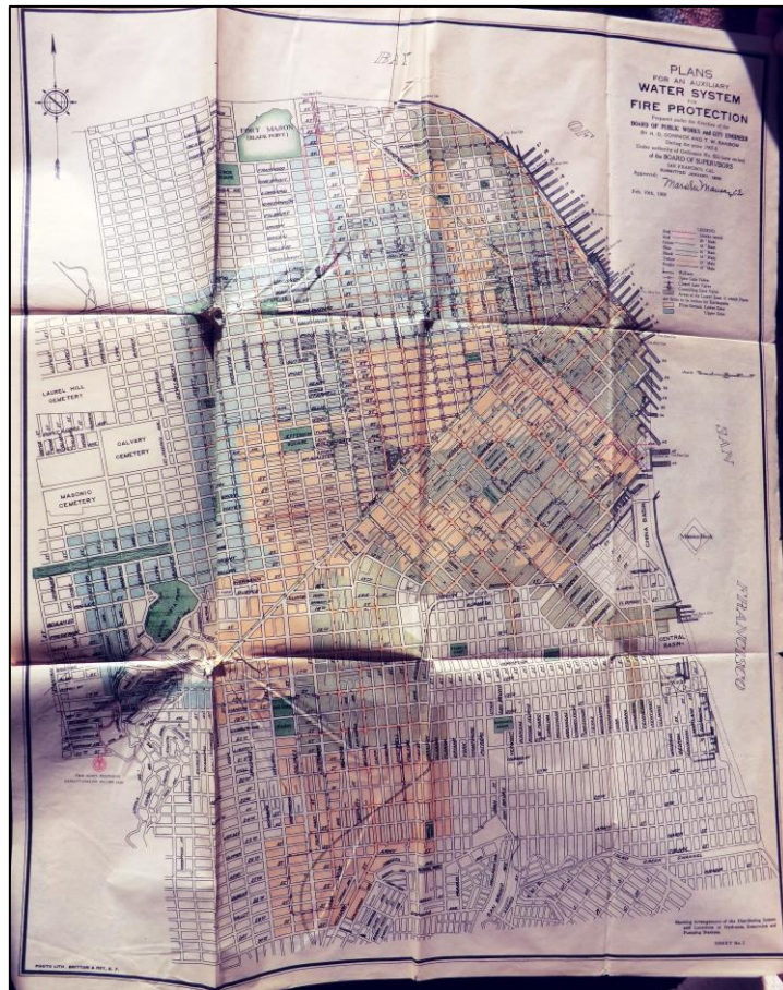
Figure 36 Manson map of 1908 showing plan for an auxiliary water system for fire protection (Manson et al. 1908)
