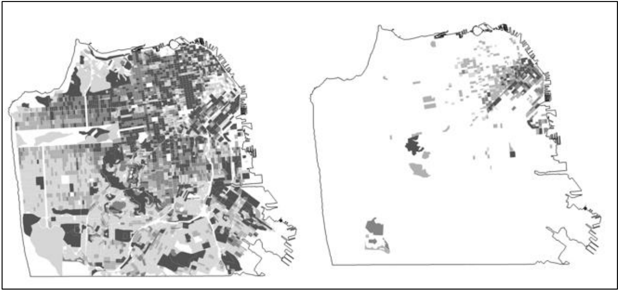
Figure 45 (left) Total Floor Area (TFA, sq. ft.) per block, for Low and Medium Rise buildings; (right) TFA per block for High Rise buildings.
