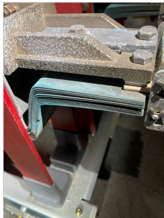
Figure 45. Photos of identified damage to Incident Cubicle and Circuit Breaker No. 56. a) Incident Insulating Board feeder side (bottom row) B-phase (middle) through-hole, b) Line side (top row) B-phase bus contact, c) B-phase vacuum bottle-top view, d) Feeder side (bottom row) C-phase breaker arm. Photo taken November 2, 2025 (courtesy PG&E).
