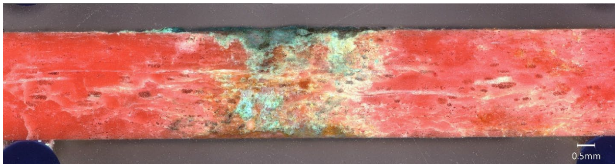
Figure 40. Mounted samples of the barrier insulating board from Cell No. 10 (bottom), showing cross section of the damaged area.
