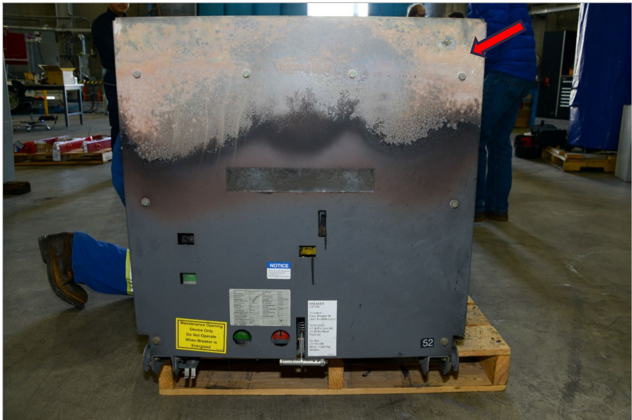
Figure 13. Discoloration and clean burn patterns on the top third of the front face on Incident Breaker No. 52 (red arrow).
