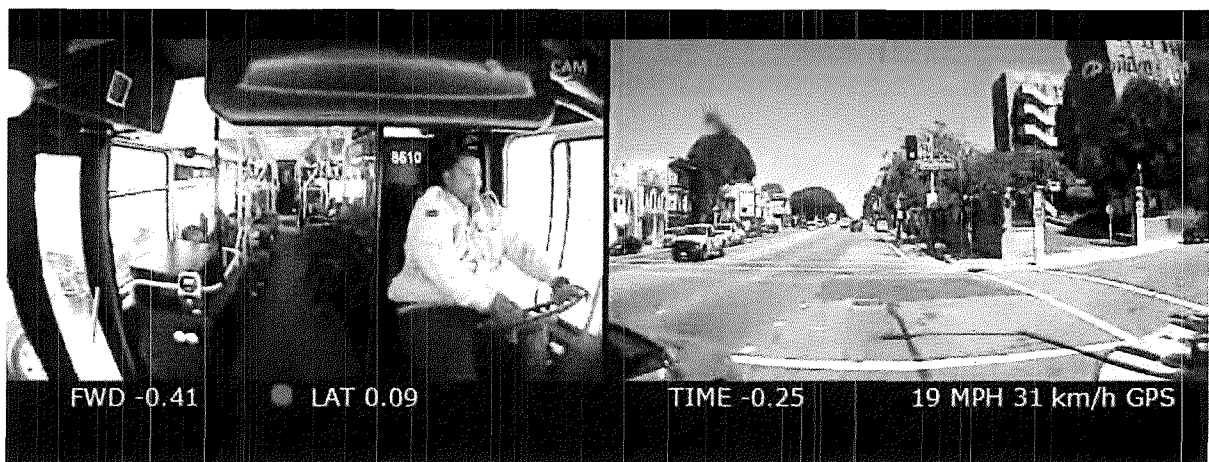
Figure 3: SFMTA's DriveCam systems record eight seconds of video before and four seconds after a fast acceleration or hard braking event.
