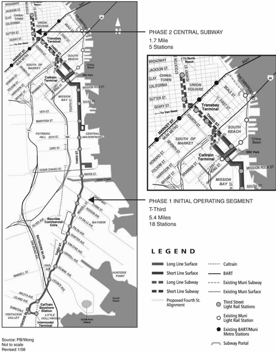
FIGURE 2-29 THIRD STREET LIGHT RAIL PHASE 1 INITIAL OPERATING SEGMENT AND PHASE 2 1998 FEIS/FEIR CENTRAL SUBWAY
