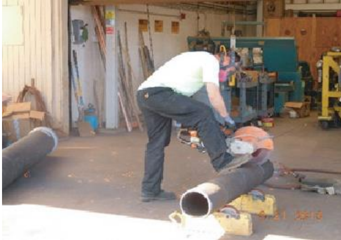
Fabrication Shop workers cut pipe at exterior of shop. Hazardous debris is not contained.
