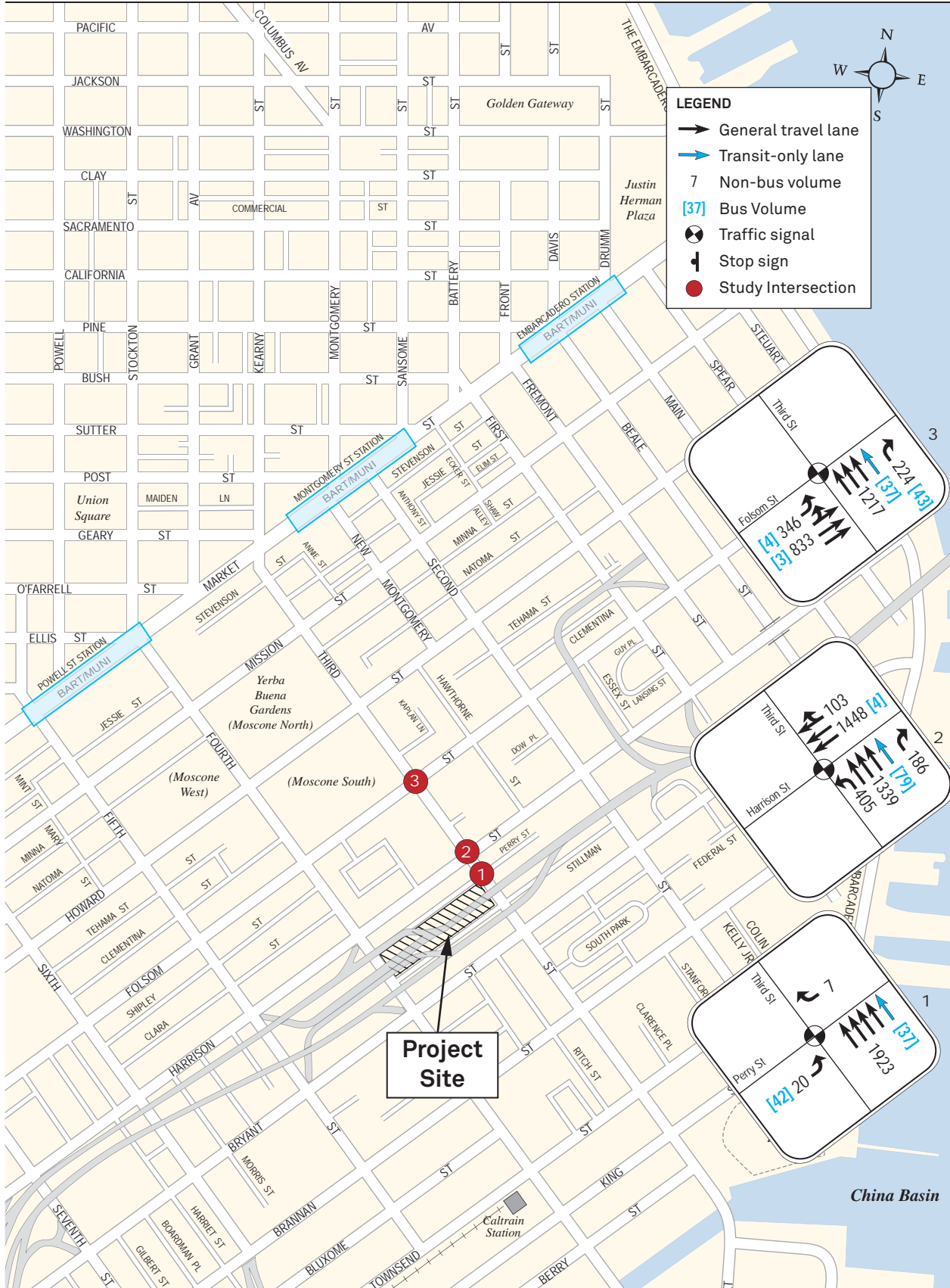
Existing Plus Project Conditions Lane Geometry and Traffic Volumes Weekday PM Peak Hour
