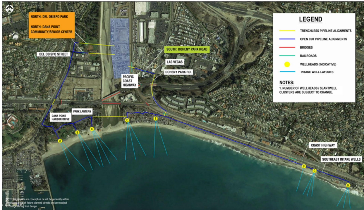
Figure 2-7: Proposed Doheny Desalination Plant Slant Well Intakes
