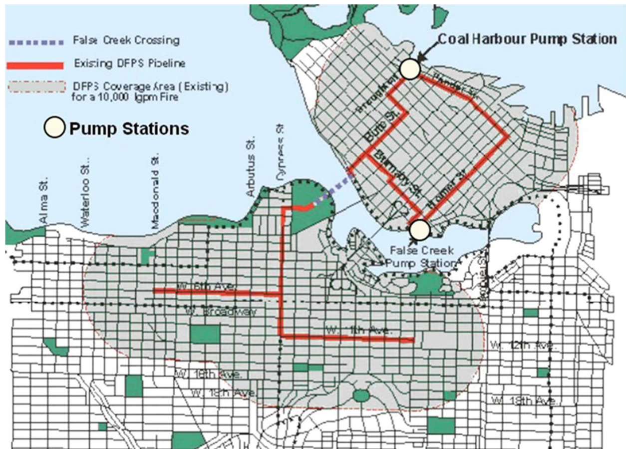
Figure 2-8: City of Vancouver, BC Dedicated Fire Protection System
