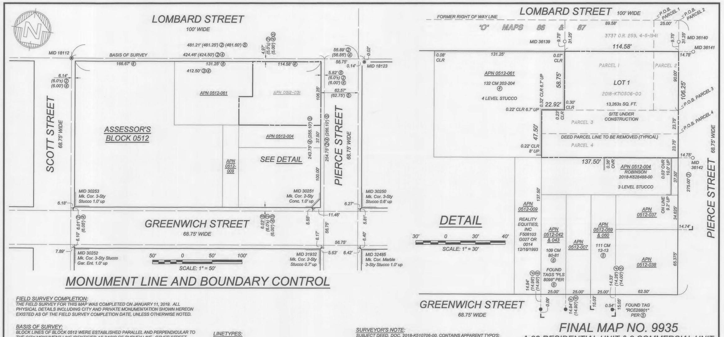
THE CITY MONUMENT LINE IDENTIFIED AS BASIS OF SURVEY LINE. OTHER STREET LINES SHOWN HEREON WERE NOT ESTABLISHED. THEY ARE SHOWN TO FACILITATE THE RECOVERY OF MONUMENT LINE REFERENCE POINTS.
