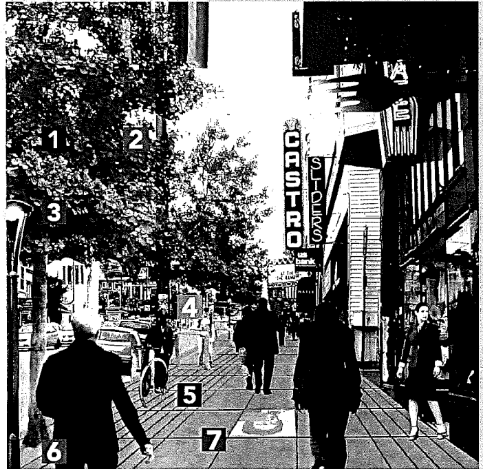
PROPOSED IMPROVEMENTS FOR CASTRO STREET 2014: 1. New Ginkgo Trees planted along curb 2. Relocated Muni and Roadway Light Poles 3. New Pedestrian-Scaled Lighting 4. Leaning Posts 5. New Bike Racks 6. Sidewalks Widened \pm 10 feet 7. Rainbow Honor Walk Plaques
