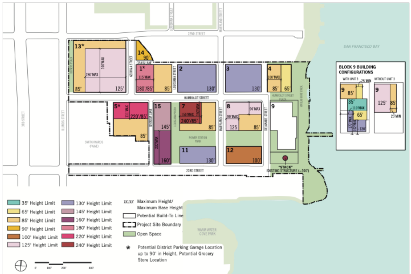
8 Figure 249.87-4: Building Heights Maximum
