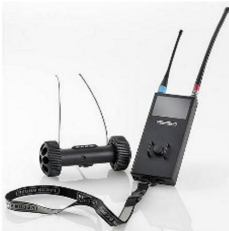
(Left) Recon Scout Robot, to be replaced by 4Sight Tactical R/C (Right).
