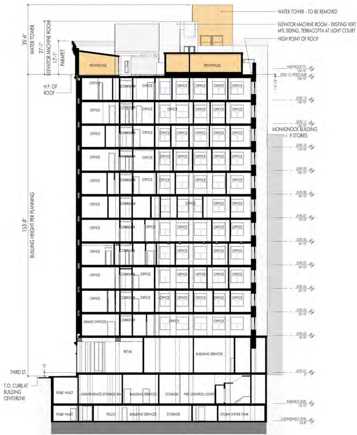
EXISTING SECTION AT CENTERLINE OF 3 RD STREET looking NORTH
