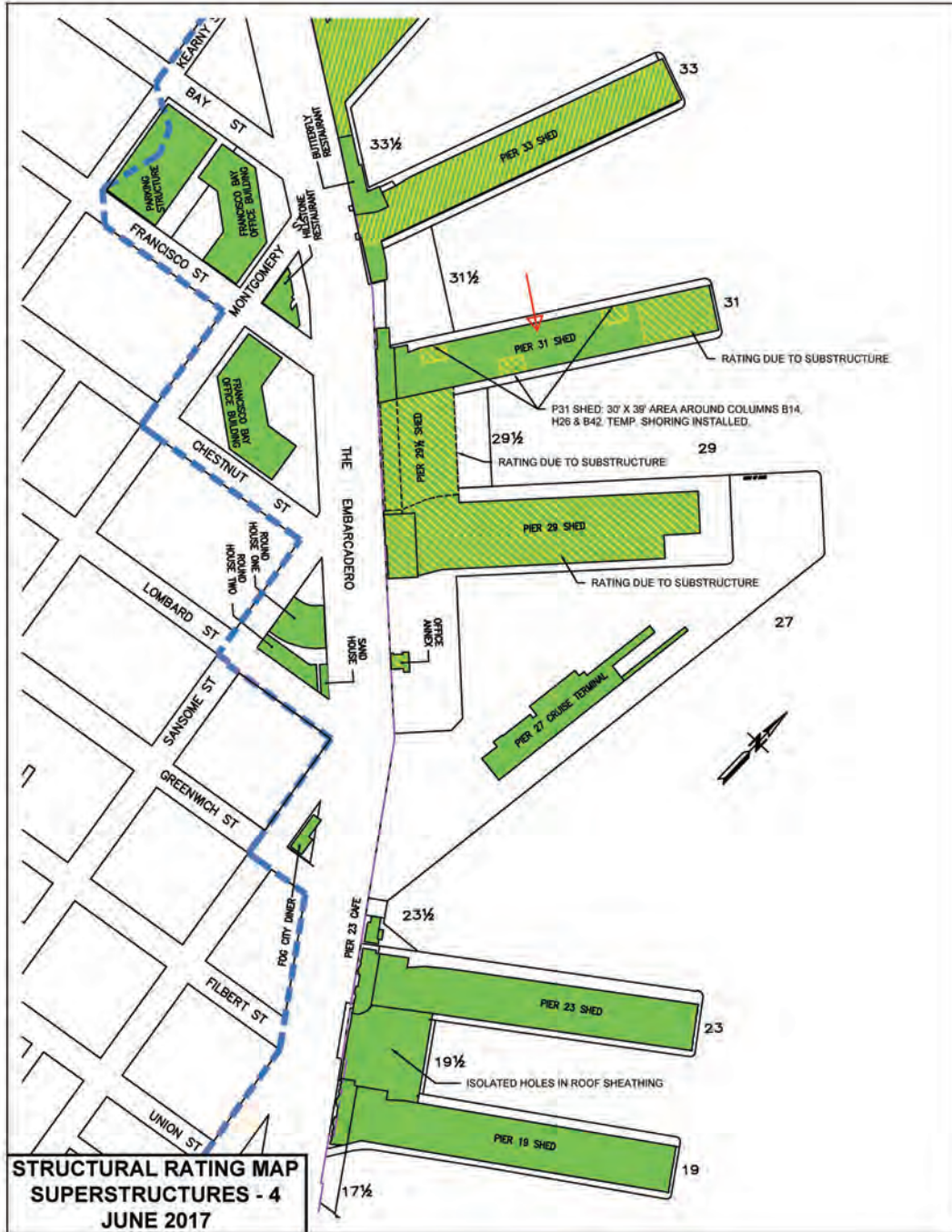
Photo 20. Superstructure rating map for Pier 31 shed. Three columns have temp. shoring and supported roof area is yellow tagged. Outer end of pier is yellow tagged due to substructure rating.
