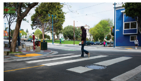
Pedestrian & transit bulb-outs extend the sidewalk into the roadway to provide safer street.
