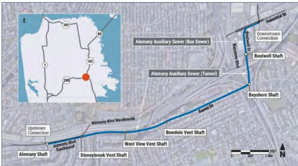
Figure 2. Project Location and Proposed Project Components
