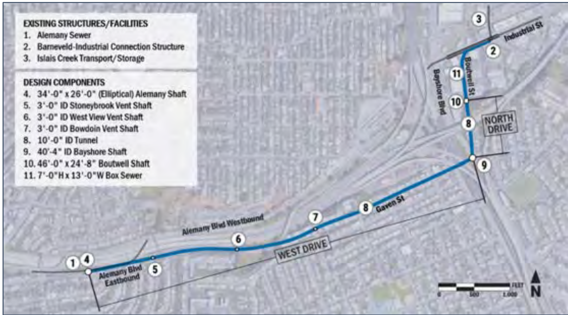
Figure 3. Existing and Proposed Project Components 2
