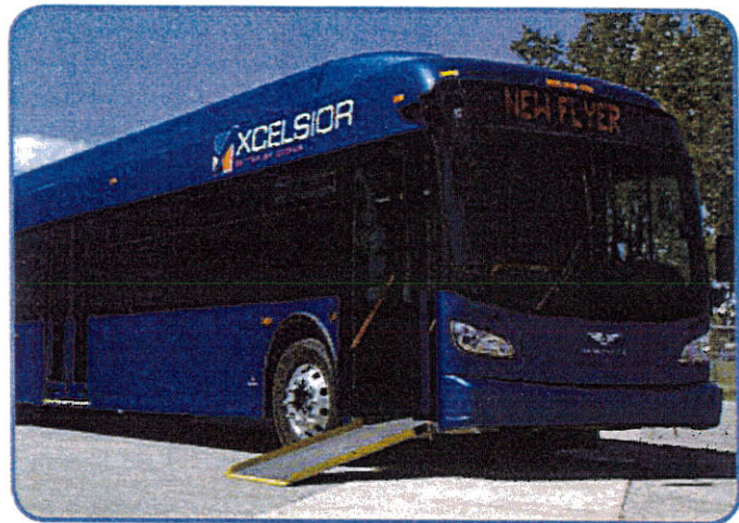
Ramp deployed at ride height street level
