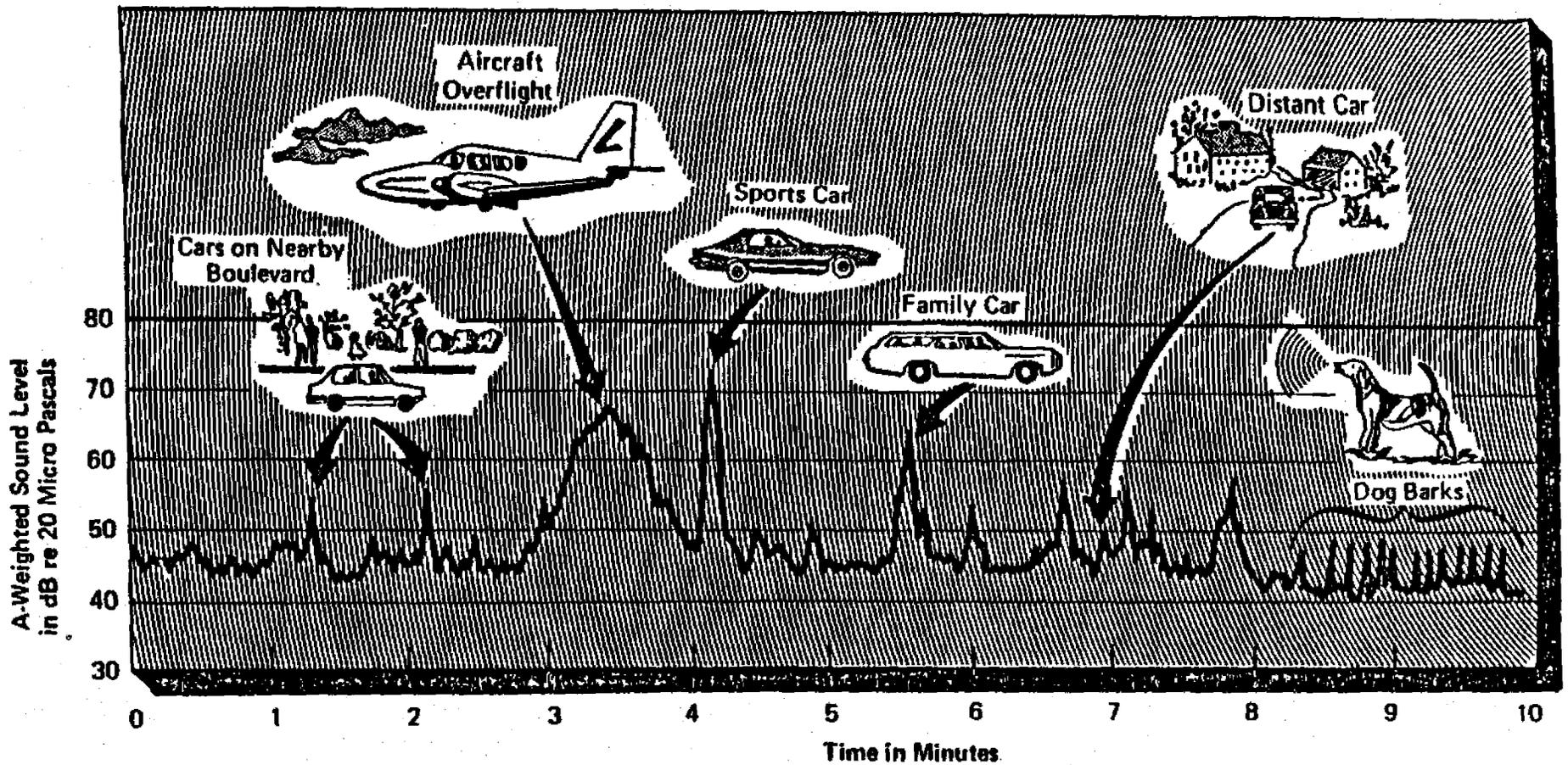
**Figure 5: Typical Outdoor Sound Measured on a Quiet Suburban Street**
