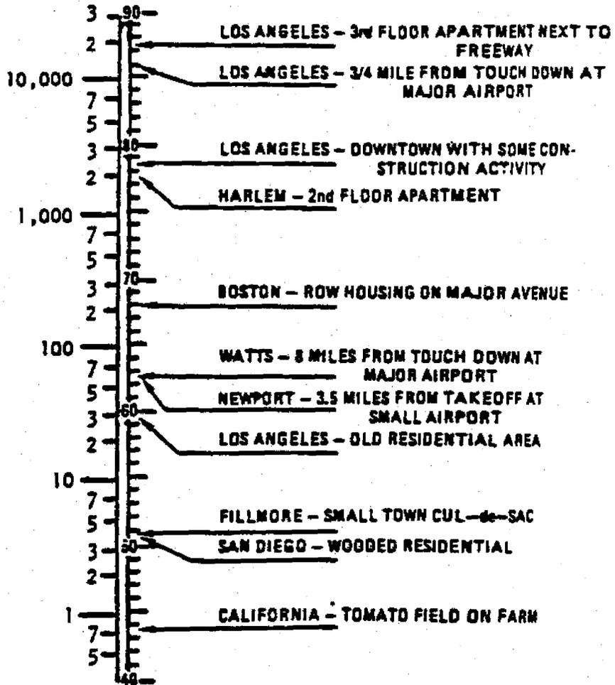
Figure 6: Examples of 24-hour Day-night Weighted Cumulative Noise Measurements with Both Day-night Weighted Sound Exposure and Day-Night Sound Level Scales
