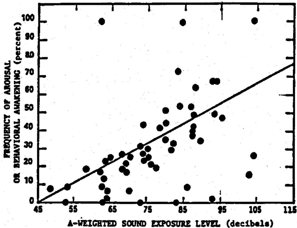
Figure 11: Probability of a Noise Induced Awakening as a Function of Sound Exposure Levels Measured Near the Sleeping Person
