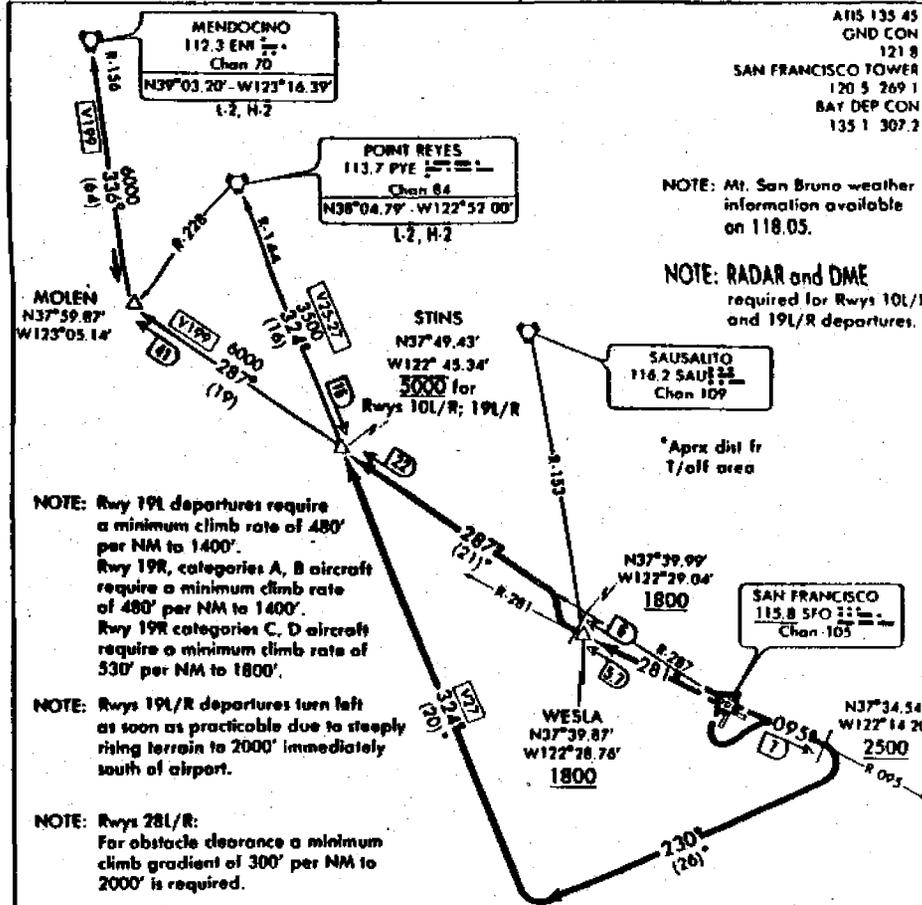
NOTE: Rwy 19L departures require a minimum climb rate of 480' per NM to 1400'. Rwy 19R, categories A, B aircraft require a minimum climb rate of 480' per NM to 1400'. Rwy 19R categories C, D aircraft require a minimum climb rate of 330' per NM to 1800'.
