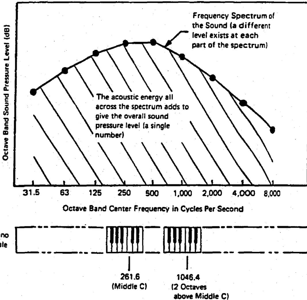
**Figure 1: Example of a Frequency Spectrum of a Sound**
