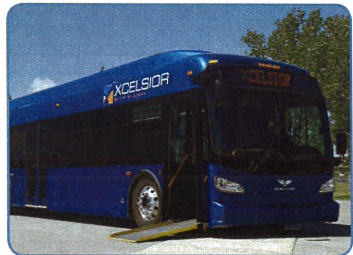
Ramp deployed kneeled (1:7) street level
