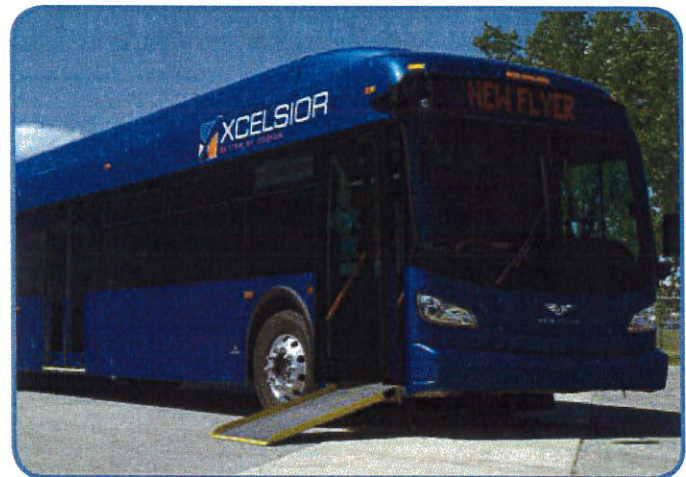
Ramp deployed at ride height street level
